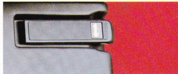
Trunk lid release from the driver's seat
