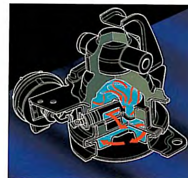
Electronically-controlled hydraulic engine mount.
