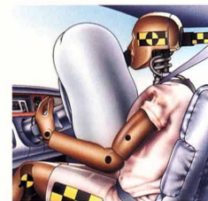
Peak inflation occurs in less than 1/25th of a second—faster than the blink of an eye. Even as the bag is inflating, some of its air is being released through the fabric to further the cushioning effect.
