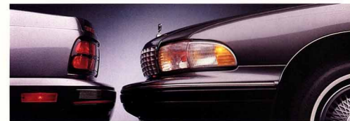
New energy-absorbing front and rear bumpers are designed to absorb a 5-mph impact without damage. These steel bumpers feature flush-fitting body-color plastic covers designed to resist minor dings and dents.
