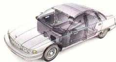
Strategic use of acoustical/sound-deadening materials helps make one of America's quietest cars even quieter.
