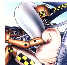
The cushion deflates rapidly as the crash ends, leaving occupant free to unbuckle safety belt and leave vehicle.
