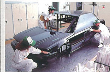
The actual-size plastic mock-up is inspected.
