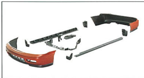
Easy-to-remove bumpers and other plastic components are marked with material ID codes to simplify recycling.
