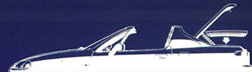
Place the roof in the hinged holder frame.
