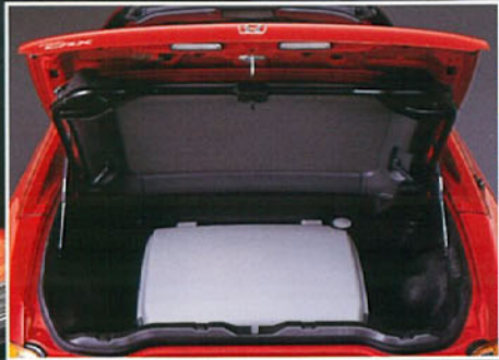
Boot space is 300 litres VDA. When the roof is stored, boot space is 236 litres VDA.
