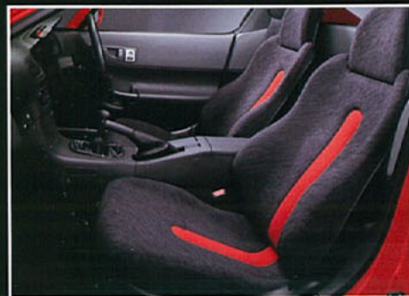
The fabric of the sporty, fully supporting CRX seats is moulded to a metal frame.
