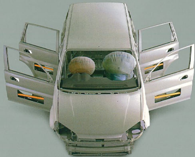
Computer designed monocoque body.
