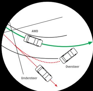
Using many elements from the famed rally-bred Mitsubishi Lancer Evolution, the QuadTec™ AWD system boasts superior roadholding and outstanding traction, which you can actually feel. Verada AWD has a refined AWD system which distributes torque evenly to all four wheels, however if it detects slip in any of the wheels the Viscous Coupling Unit regulates the torque to ensure that the car continues to corner efficiently, maintaining stability and power.
