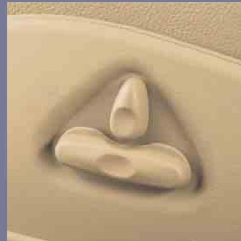
10 way power adjustable driver seat and 8 way power adjustable passenger seat.
