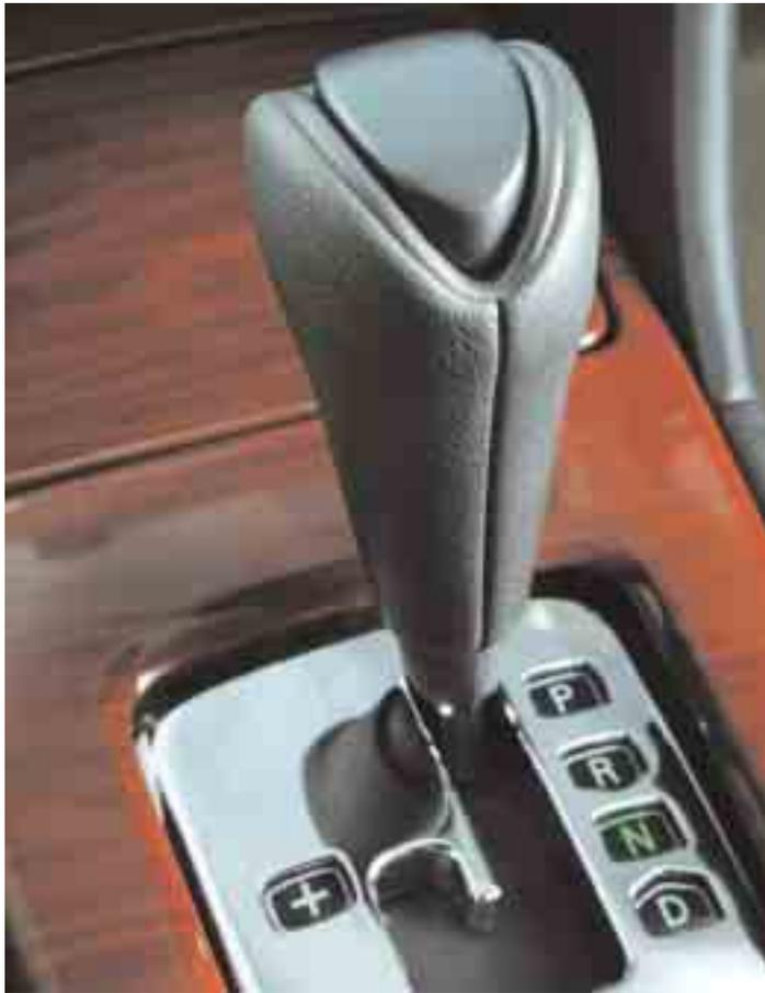
'SPORTS MODE' sequential gear shifting makes Verada's 5 speed INVECS II 'Smart Logic' automatic transmission even more flexible. When the shift lever is moved sideways 'SPORTS MODE' is engaged letting the driver push the lever forward to go up a gear or pull it back to shift down a gear. So you can have the benefits of a normal automatic for around the city, with a more responsive clutchless manual for open road driving.
