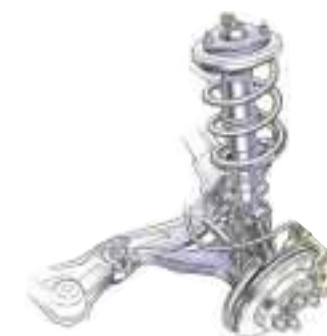
Honda's refined strut has created a much improved independent front suspension.
