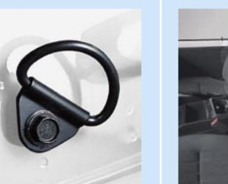
A cargo protection bar and cargo tie down rings, prevent loose loads from moving around in transit.
