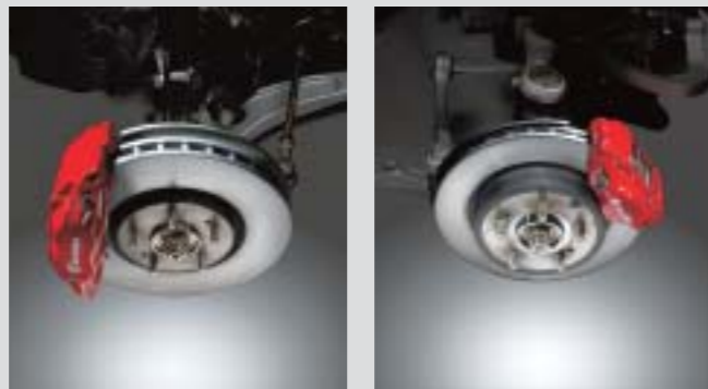
REAR 17" DISC BRAKES WITH 4-POT BRAKE CALLIPERS
