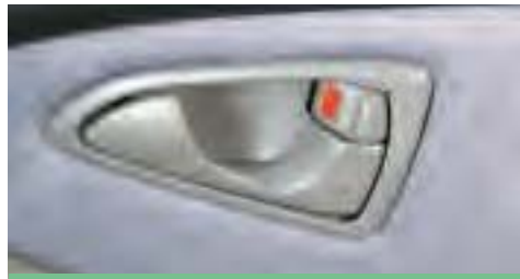
EMERGENCY DOOR UNLOCK - FRONT & SIDE
