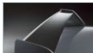
Rear Spoiler Extension - Dark Grey Rear downforce approximately +4kgf@180km/h
