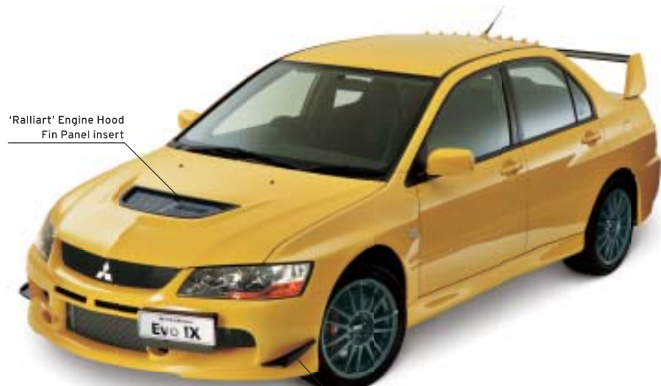
Front Bumper Side Spoilers Front downforce approximately +4kgf@180km/h
