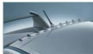
Vortex Generator - Body Coloured Rear downforce approximately +2kgf : Aerodynamic Drag (CD) : -1.1%@180km/h
