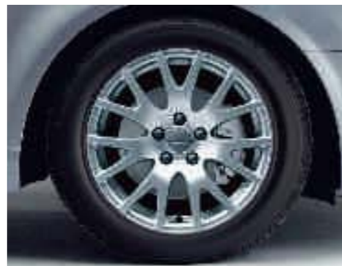
Lightweight forged aluminium wheels in 7-Y-spoke styling, size 7.5 J x 17 with 225/45 R 17 tyres
