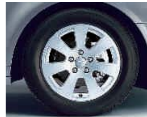
Cast aluminium wheels in 7-arm styling, size 6.5 J x 16, with 205/55 R 16 tyres (exclusively for Ambiente)
