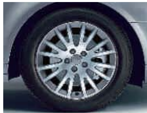
Cast aluminium wheels in 16-spoke styling, polished, two-tone, size 7.5 J x 17 with 225/45 R 17 tyres
