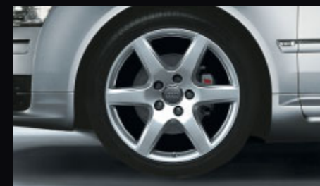
Winter wheels in 6-arm styling 1 , with PAX run-flat system, 235 x 500 (equivalent to 19 inches) with 235/690 R 500 tyres, permitted top speed 210 km/h; suitable for fitting with snow chains
