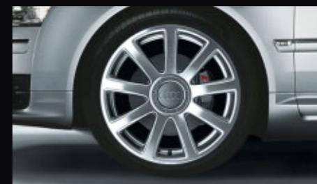
Forged aluminium wheels in 9-spoke styling 2 , high-gloss polished finish, single-colour, size 9 J x 20 with 275/35 R 20 tyres
