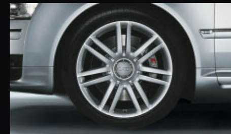
Cast aluminium wheels in S styling, size 9 J x 20 with 265/35 R 20 tyres
