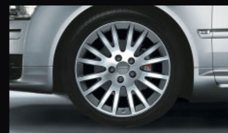
Winter wheels in 16-spoke styling, size 8 J x 19 with 235/45 R 19 tyres, permitted top speed 210 km/h; suitable for fitting with snow chains
