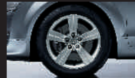
Cast aluminium wheels in 5-arm trapezoidal styling, size 8 J x 17 with 225/50 R 17 tyres
