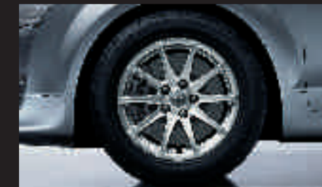
Cast aluminium winter wheels in 10-spoke star styling, size 7 J x 16 with 225/55 R 16 H tyres, permitted top speed 210 km/h
