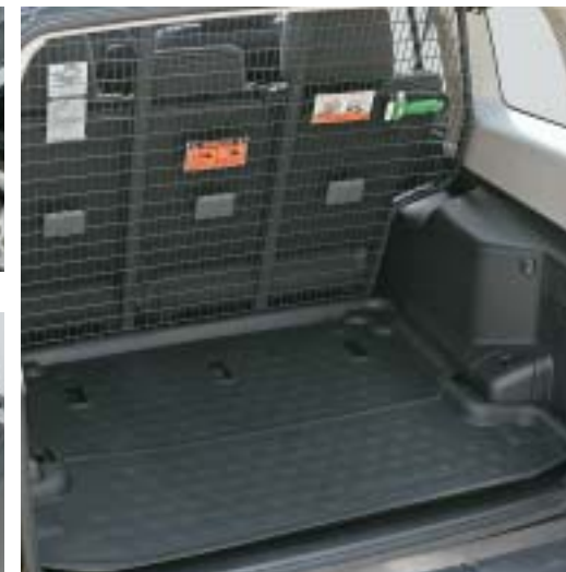
CARGO BARRIER AND TRAY LINER
