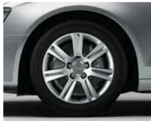
Cast aluminium wheels, 7-arm structure design, size 7.5 J x 17 with 225/50 R 17 tyres
