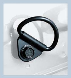
A cargo protection bar and cargo tie down rings, prevent loose loads from moving around in transit.
