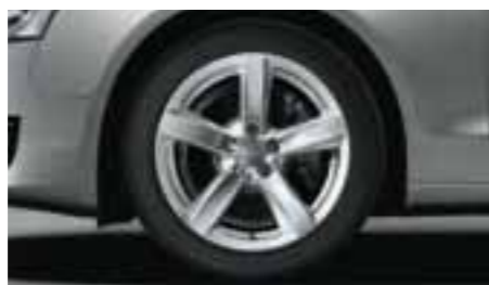
Cast aluminium wheels, 5-arm dynamic design, size 8.5 J x 18 with 245/40 R 18 tyres
