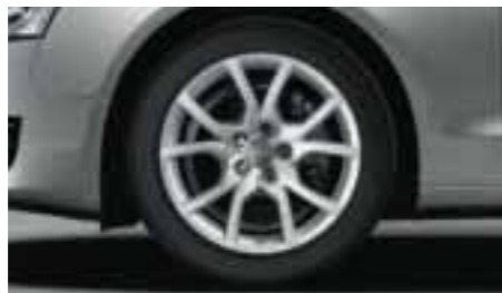
Cast aluminium wheels, 10-spoke V design, size 8.5 J x 18 with 245/40 R 18 tyres
