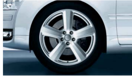
Audi exclusive cast aluminium wheels, in 5-arm design, size 9 J x 19 with 255/40 R 19 tyres. From quattro GmbH
