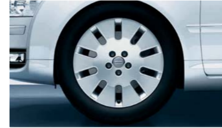
Winter wheels, in 10-arm design, size 7.5 J x 18 with 235/50 R 18 tyres, permissible top speed 240 km/h, can be fitted with snow chains
