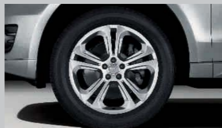
Audi exclusive cast aluminium wheels, 5-double-spoke offroad design, size 8.5 J x 20 with 255/45 R 20 tyres, including wheel arch strips. From quattro GmbH
