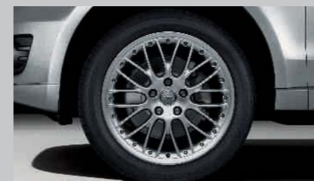
Audi exclusive cast aluminium wheels, 20-spoke design, two-piece, size 8.5 J x 20 with 255/45 R 20 tyres, including wheel arch strips. From quattro GmbH
