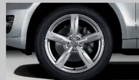
Cast aluminium winter wheels, 5-arm design, size 8.5 J x 20 with 255/45 R 20 tyres, cannot be fitted with snow chains, including wheel arch strips, permissible top speed 240 km/h
