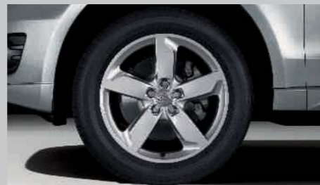
Cast aluminium wheels, 5-arm design, polished, size 8 J x 19 with 235/55 R 19 tyres
