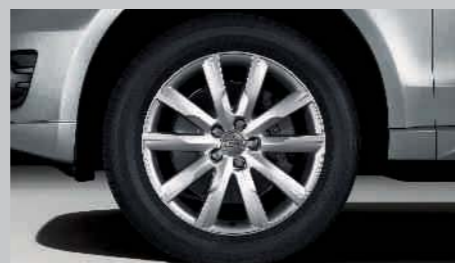
Cast aluminium wheels, 10-spoke design, size 8 J x 19 with 235/55 R 19 tyres
