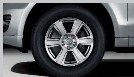
Cast aluminium wheels, 6-arm design, size 8 J x 17 with 235/65 R 17 tyres
