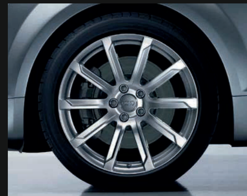
Audi exclusive cast aluminium wheels, 10-spoke design, size 9 J x 18 with 245/40 R 18 tyres. From quattro GmbH
