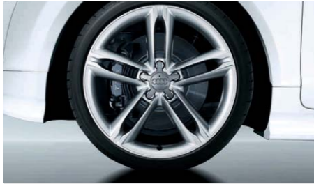
Cast aluminium wheels, 5-parallel-spoke star design, size 9 J x 19 with 255/35 R 19 tyres
