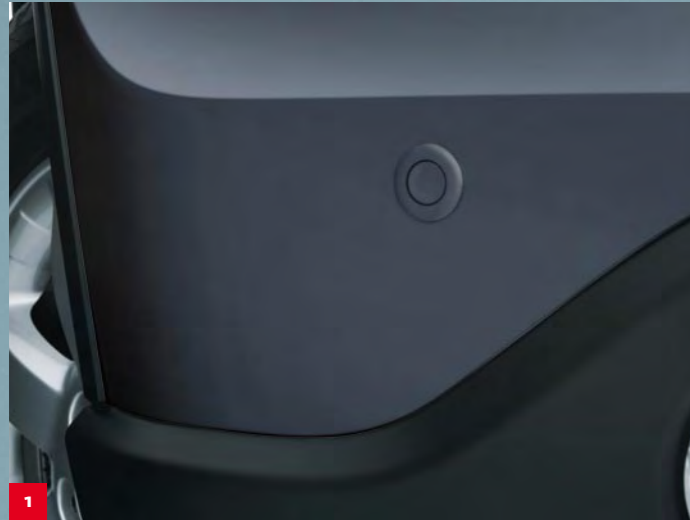
Figure 1. Front Corner Park Assist Sensor Range:
