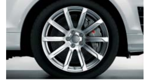
Cast aluminium winter wheels, 10-spoke design, size 10 J x 20 with 275/45 R 20 tyres, can be fitted with snow chains, permissible top speed 240 km/h
