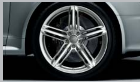
Cast aluminium wheels in 5-segment spoke design, 9.5 J x 20 with 275/35 R 20 tyres
