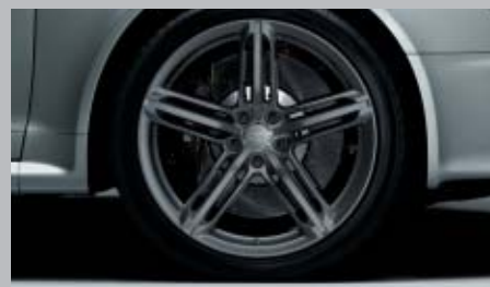
Cast aluminium wheels in 5-segment spoke design, titanium look, 9.5 J x 20 with 275/35 R 20 tyres
