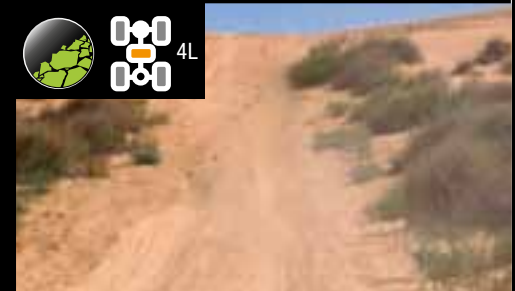
4LLC (4WD Low Range w/ Locked Centre Differential)
