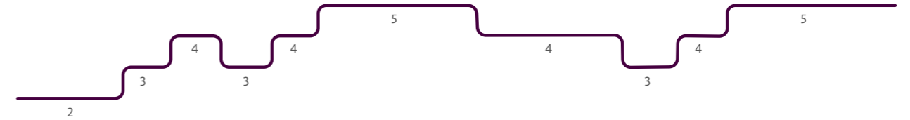
Typical 'gear hunting' without Grade Logic Control
