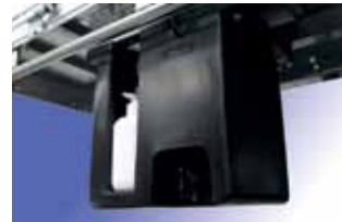
Water Tank (A) (S)
