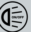
Auto lights on/off Monitors outside light levels and turns headlamps on or off accordingly. (Neo and Maxx only.)
