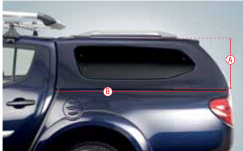
Sports Style – Dimensions: A – 565mm, B – 1506mm, C – 1590mm, D – 1180mm
