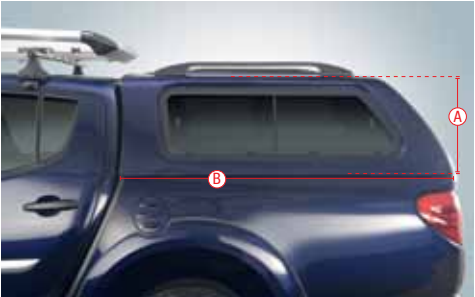
Trade Style – Dimensions: A – 550mm, B – 1506mm, C – 1590mm, D – 1200mm
