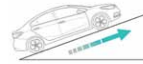
Hill-start Assist Control (HAC) By maintaining brake grip until you press the accelerator, HAC prevents the vehicle from dangerously rolling backwards when pulling away from a standstill on an incline.
