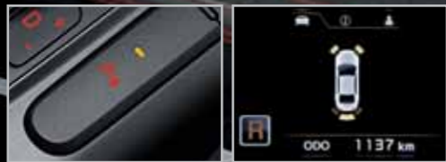
Front corner and rear parking assist system Activated by a switch on the floor console, (on A/T models, M/T models have a switch on the lower dash), the standard front corner and rear parking assist system shows the distance between the car and any obstruction by means of a graphic on the cluster. (Some exterior colours come with black sensors).
