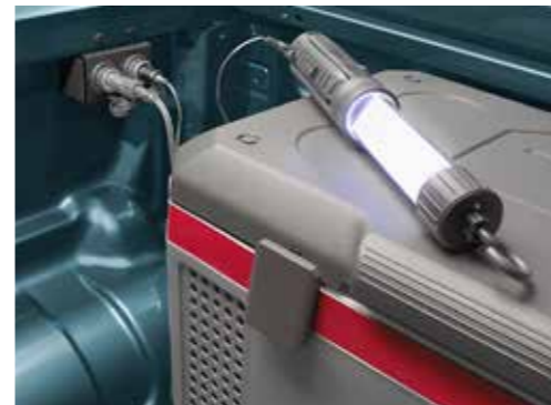
12 volt auxiliary sockets Contains two 15 amp sockets to provide power to small electrical items. (Utilities only)
