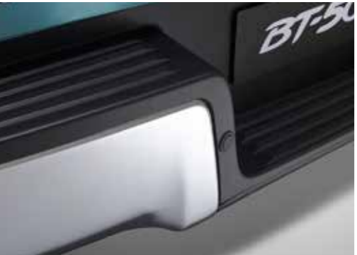
Reverse parking sensors Advanced sensors use warning tone to make parking easier, even with a tow bar. (Utilities only)
