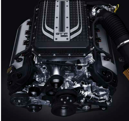
Boss 5.0 litre, supercharged DOHC 32 valve all-aluminium V8. Maximum power (DIN) 351kW @ 6000rpm^ Maximum torque (DIN) 570Nm @ 2,500-5,500rpm^
