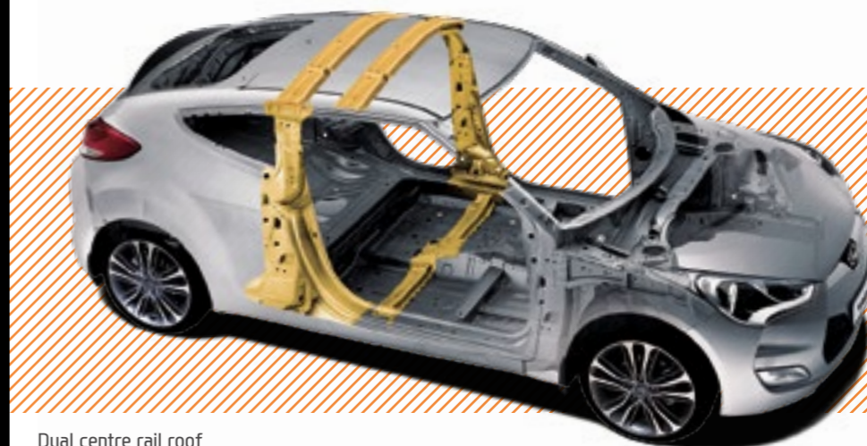
Dual centre rail roof To provide further protection in a collision, both the dash cross member and side members, as well as the roof structure and pillars are made from reinforced sheet steel.
