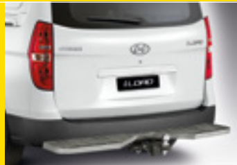
Technician Step with Grab Handles
