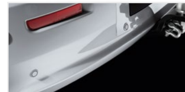
Rear Parking Assist Sensors
