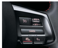
SI-Drive steering wheel controls CVT variants
