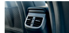
Rear cooling/heating vents
