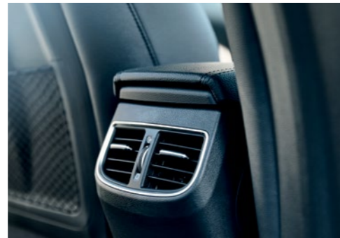
Rear cooling/heating vents 1
