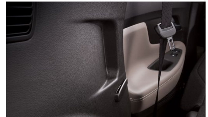
3rd row grip handles 1 Handles in the 3rd row help occupants enter and exit the vehicle with ease.
