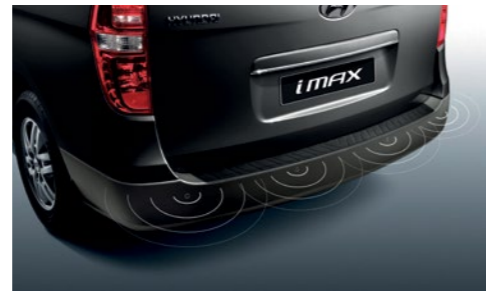
Rear parking assist system
