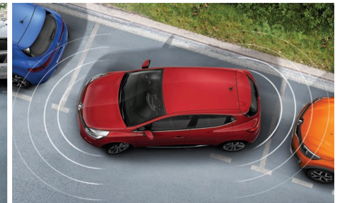
The hands-free parking system has 12 sensors placed on the front, rear and sides to detect a spot with adequate dimensions to park your vehicle.
