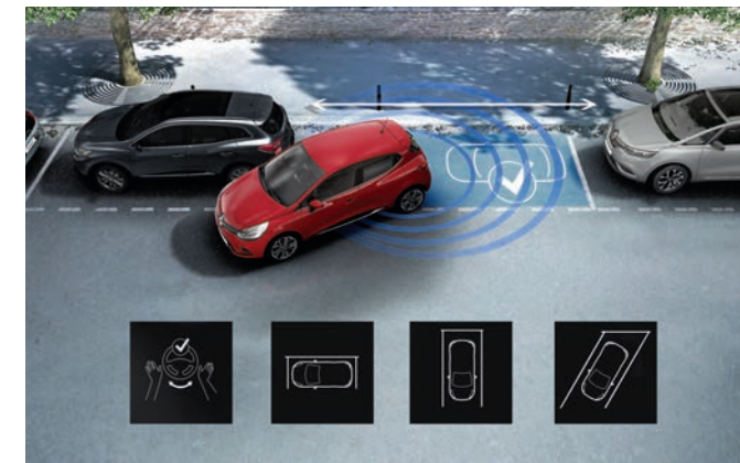
Hands-free parking (with R-LINK)** Tight spots have never been easier to handle with hands-free parking. The system assesses the available space and defines the trajectory. Let it take control of the steering whilst you simply control the speed for hassle-free parking.
