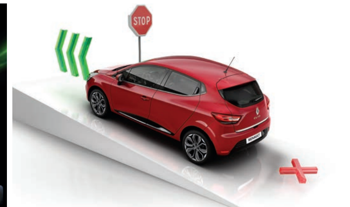
Hill Start Assist (HSA) When starting the vehicle on a hill the brake pressure is automatically maintained for two seconds, giving the driver time to manoeuvre.
