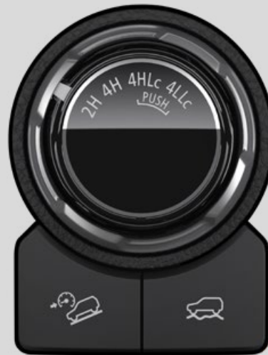
4HLC (4WD High Range with locked centre differential) For low-grip surfaces like unsealed roads and sand.
