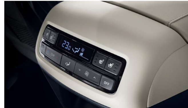
Three-zone climate control system 1 Dual-zone for the driver and front seat passenger (which means you can both enjoy different climate settings), temperature and control settings in the 2nd row and air vents in the 3rd row.
