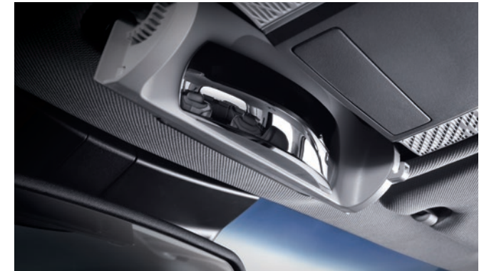
Rear conversation mirror Displays vision of passengers in the 2nd and 3rd rows to the driver, allowing parents to safely keep an eye on the little (or not so little) ones in the back.
