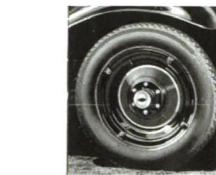
New, larger, full balloon Tyres 5.00 ins. x 19 ins. Actually 5-2/10 in. sectional diameter. The reduced wheel size adds to appearance—larger tyre improves riding.
