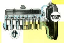
Cooling . . . The Holden engine operates efficiently regardless of outside temperature because water circulation is controlled by an automatic all-weather thermostat. Full length water jackets completely surround all cylinders and jet cooling prolongs the life of valves and seats.
