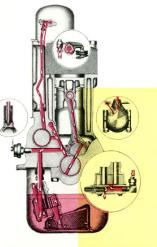
Lubrication . . . 100% full pressure metered-flow lubrication is another feature which helps in the splendid performance and general economy of the Holden engine.
