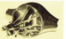
Holden's differential has a specially stiffened carrier to ensure long, trouble-free service. The low pinion engagement of the Hypoid Rear Axle contributes to Holden's low, sleek lines.
