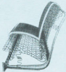
Holden front and rear seating, with proven Z type, non-sag seat springs, is soft, comfortable. The front seat is designed to give excellent vision.
