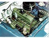
Money-saving performance ... The famous Holden O.H.V. engine develops 70 gross b.h.p. with a compression ratio of 6.8 to 1, giving lively acceleration, with fine top goor and hill climbing performance and remarkable economy. A new 12 volt electrical system provides more efficient lighting, storting and ignition performance.
